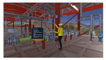
Figure 8 - Monitor editable building information through selection and expression-based styling on 3D data
